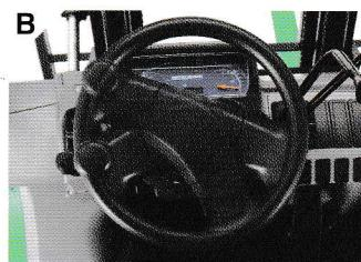
**Power Steering With 100% Standstill Steering**
