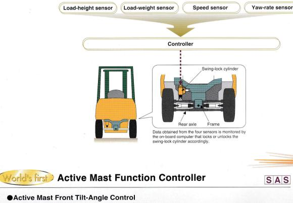
Computer-control of the mast's front tilt angle, according to the height and weight of the load, lowers the risk of the load falling or the likelihood of the vehicle overturning as a result of operator error.
