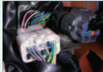
Water-Resistant Connectors Connectors for most electrical components are highly water-resistant, increasing the reliability of the electrical system.
