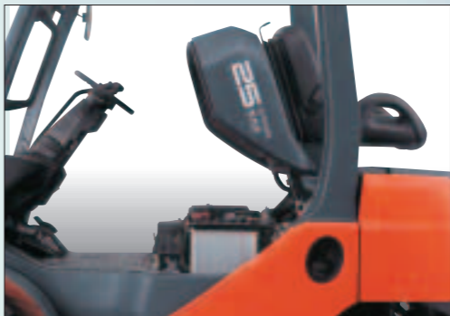
Engine Hood The wide-opening engine hood provides easy access for inspections or servicing.
