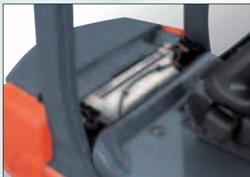
Radiator Cover No tools are needed to remove the radiator cover. The fasteners can easily be turned by hand to enable quick inspections or servicing.
