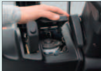
Brake Fluid Simply lift up the cover on the panel to check the brake fluid.
