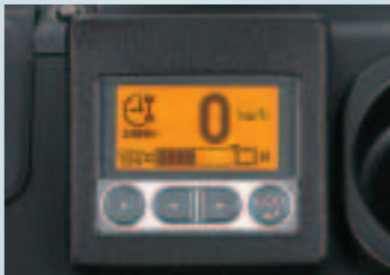
Scheduled-Maintenance Hour Warning Indicator (Multifunction Display OPT ) When the set time for maintenance is reached, this feature provides visible and audible notification.
